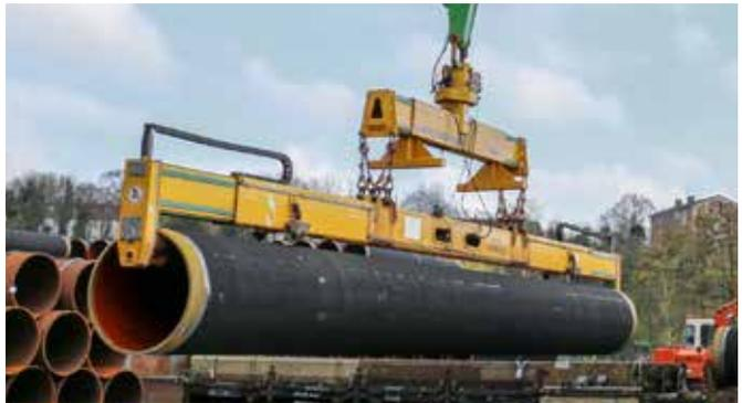
Quick change system with lifting beam
