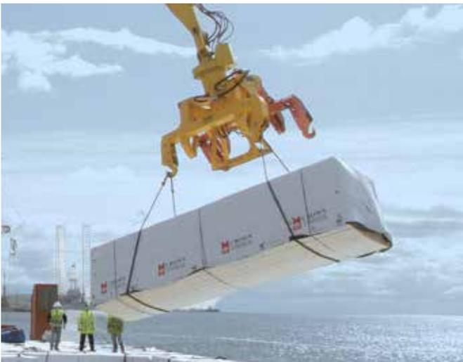
Timber spreader / wooden pallet loading
