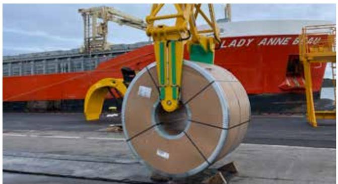
Spreader for steel coils
