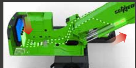
The nearly constant force transmission throughout the cylinder cycle supports the next boom lift
