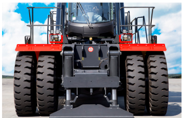
Stabilizers Can Be Deployed to Provide Additional Capacity (Standard)
