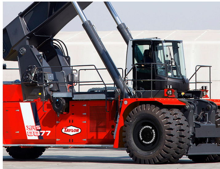
Center mounted sliding cabin (tracks to front of machine)
