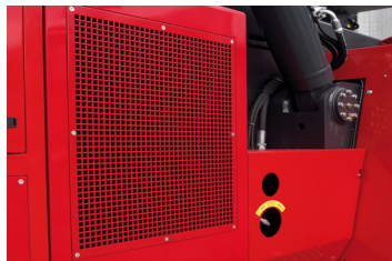
Large Hydraulic & Transmission Oil Cooling System
