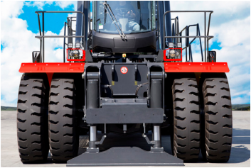
Stabilizers Can Be Deployed to Provide Additional Capacity
