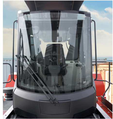
Fully Enclosed 2 Door Cab with Multiple Climate Control Configurations Available (featured cab is shown with available options)
