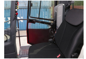
Fully Adjustable Mechanical Seat (Standard)
