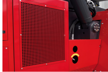
Large Hydraulic & Transmission Oil Cooling System
