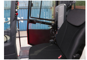
Fully Adjustable Air Suspended and Heated Seat (Standard)
