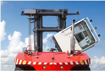
Tilting Cab for Easy Access to Drive Train & Hydraulics
