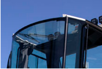
FOPS Compliant Top Glass for optimal Driver Visibility (Standard)
