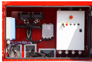
All-Weather Proof Connectors and Junction Boxes (Standard)
