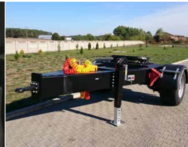
Dolly-type trolley enables to move MPB 20.72 with truck or tractor
