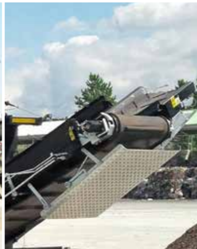
Magnetic roller for removal of ferrous metals may be mounted on rear and side discharge conveyors.
