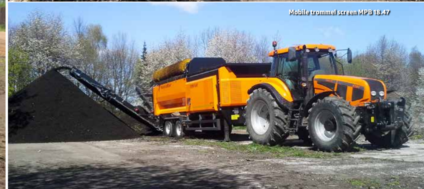
PRONAR MPB 18.47 trommel screen sieving waste after biological stabilisation.
