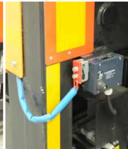
Side guards protection system stops machine when side shields are unauthorized opened
