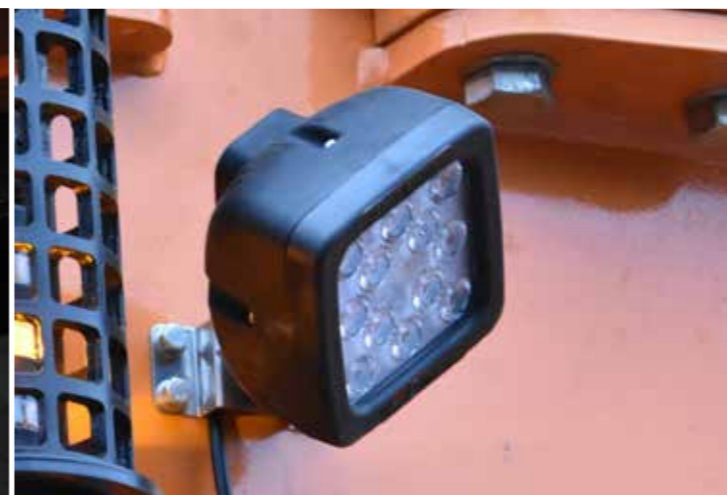
Working area additional lighting
