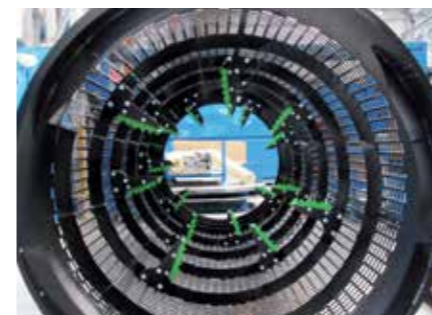
Optional knives for trommels for tearing refuse bags
