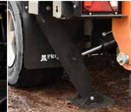
Hydraulic support legs improve machine stability during operation.
