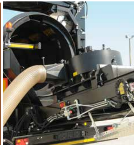
Air separator for removal of paper and light plastics.
