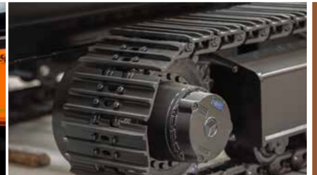
Crawler track drive allows for free movement of the machine. Two track speeds allow precise adjustment of machine's position for optimum efficiency. Tracks designed by the reputable brand of Keestrack.
