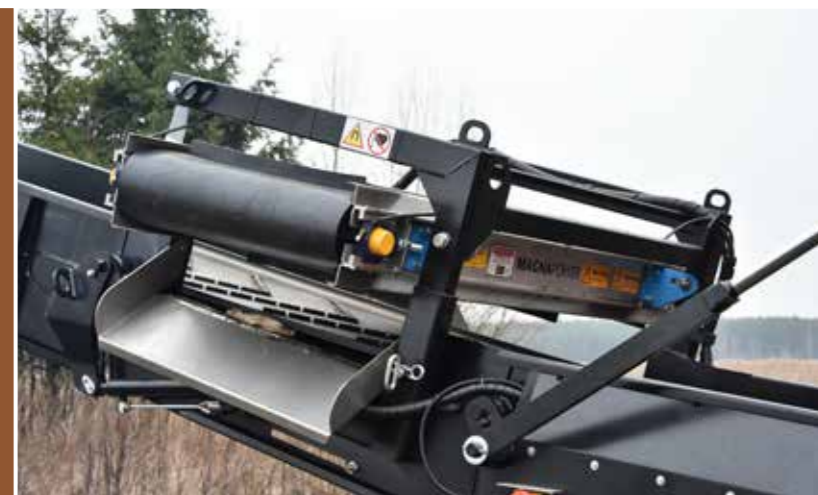
Magnetic separator for extraction of ferromagnetic materials.
