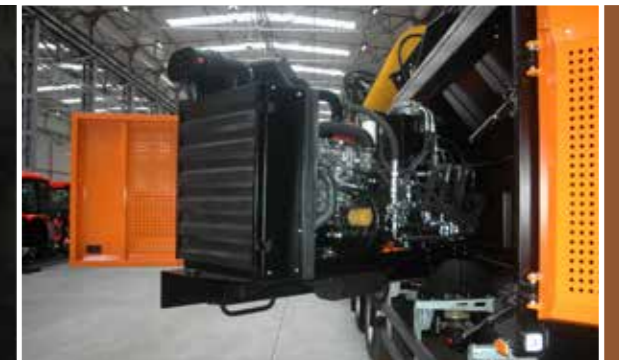
The engine and hydraulic system are mounted on a pull-out frame which provides easy access for maintenance.
