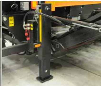
Hydraulic support legs improve stability of the machine on uneven ground.
