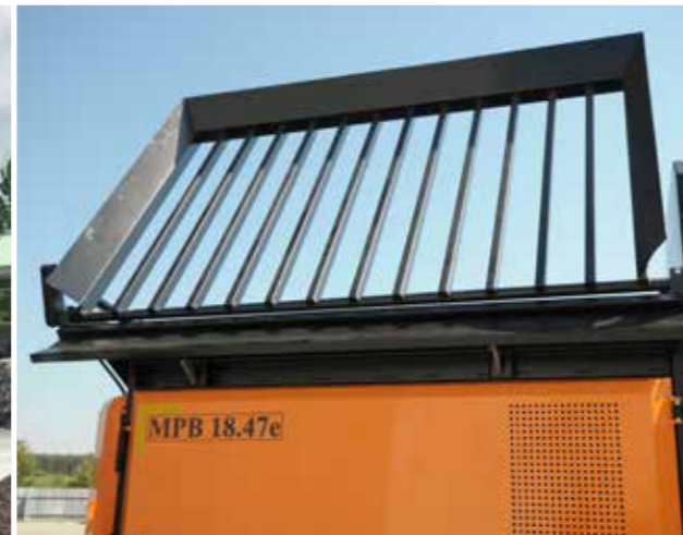
Hydraulic tipping grid for removal of large objects to prevent damage to the trommel drum.
