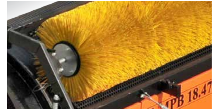
Hydraulically raised and lowered trommel cleaning brush.
