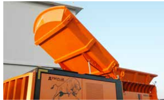
Thanks to remote control a hydraulically raised chute increases machine output and operator's work comfort.
