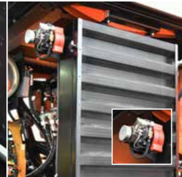
Hydraulic oil radiator cleanfix system for optimal and uninterrupted operations.
