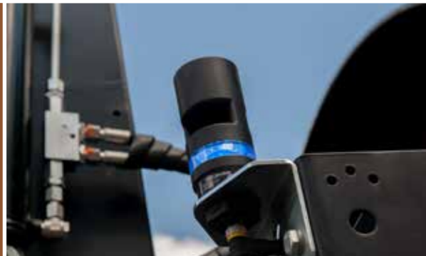
Beacon light signals the work/drive mode
