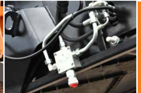
Conveyor belt speed rate adjustment
