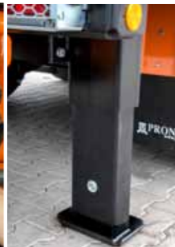
Hydraulic support legs ensures stability of machine
