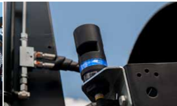
Beacon light signalises work/drive mode
