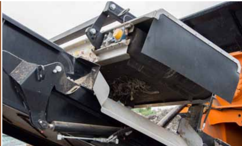
Magnetic separator for extraction of ferromagnetic materials.
