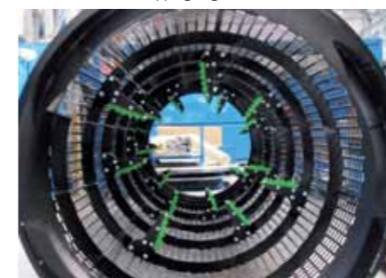
Screwed knives for ripping bags with waste*
