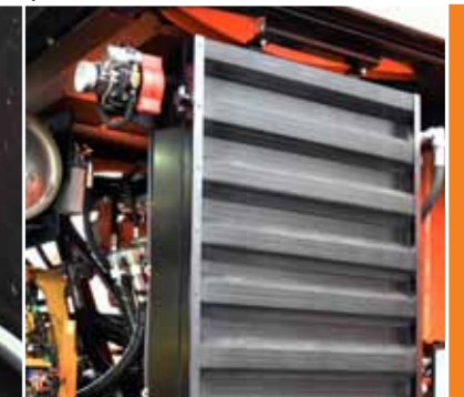
Cleanfix systems automatically clean engine and oil hydraulics radiators
