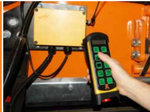
Remote control for basic machine operating functions
