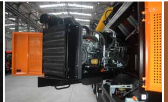
The engine and hydraulic system are mounted on a pull-out frame which provides easy access for maintenance
