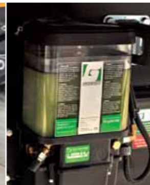
Central lubrication system ensures good greasing of the most important parts of the machine. Two sizes available
