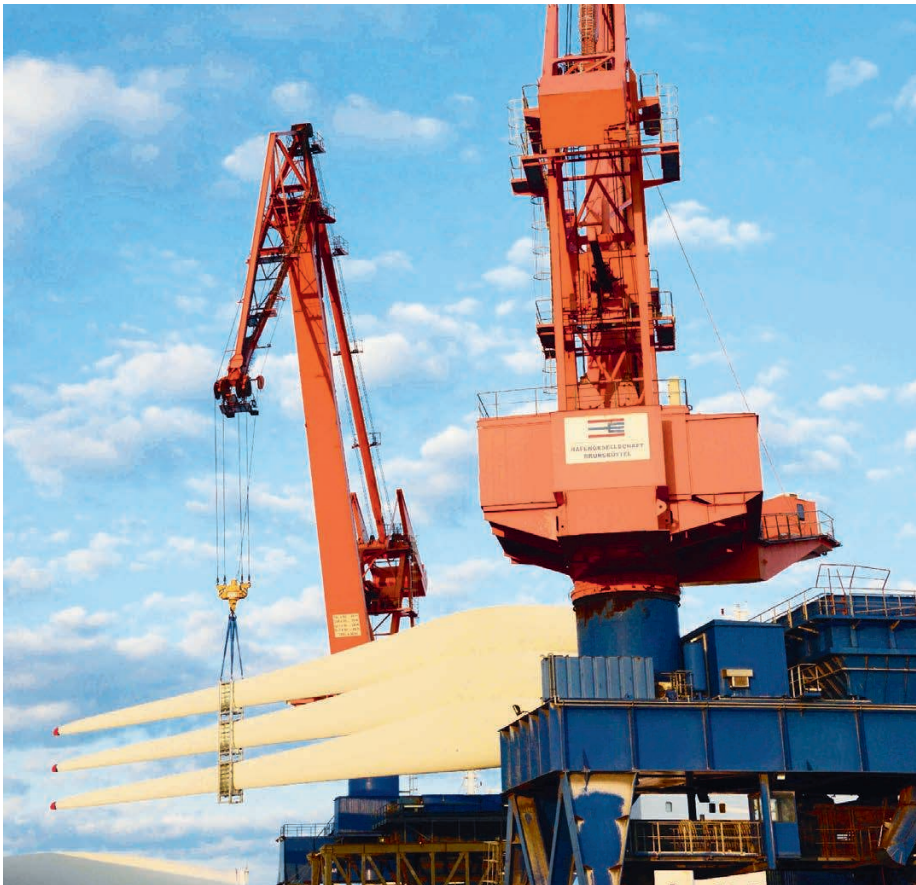
↑ Heavy load handling of parts for wind turbines in tandem operation
