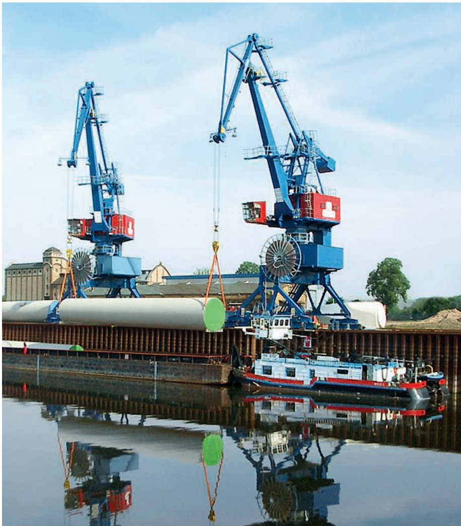
↑ Loading parts for wind turbines in tandem operation
