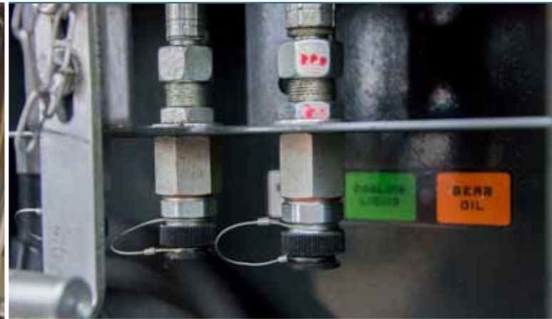
Central system for exchange of operating fluids has been placed on the left and right sides of the machine
