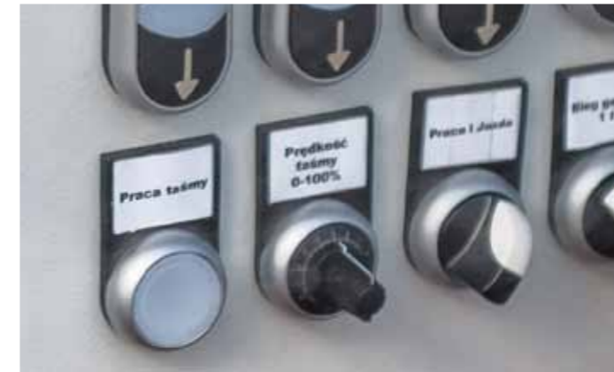
Smooth speed regulation of the feeding belt
