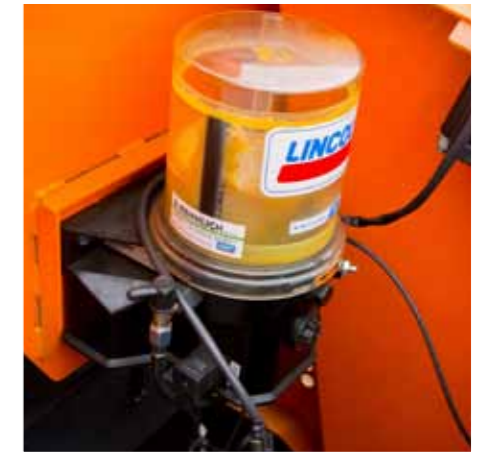
Central lubrication system improves the comfort of work and ensures the continuity of lubrication of the most important points of the machine, extending its working life
