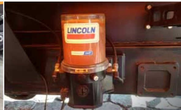
Central lubrication system ensures good greasing of the most important parts of the machine. Two sizes available
