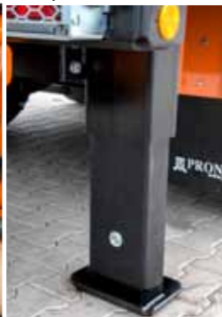
Hydraulic support legs ensures stability of machine
