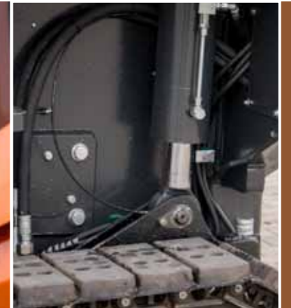
The Windrow Turner with the working shaft has the possibility of lifting 35 cm
