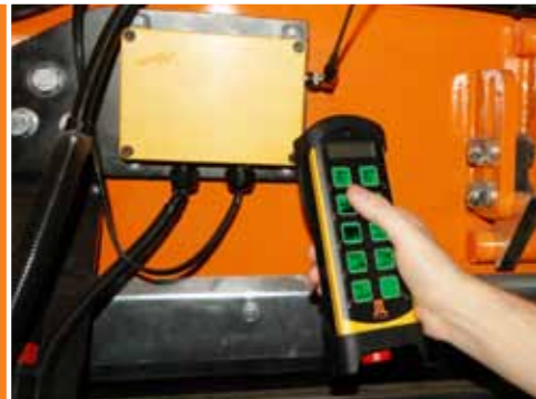
Remote control for basic machine operating functions
