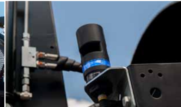
Beacon light signalises work/drive mode
