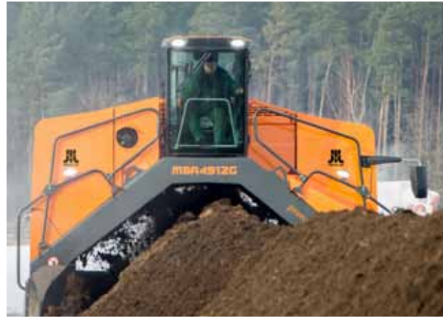
Four independently adjustable work lamps on both front and back allow to work after dark and in difficult lighting conditions
