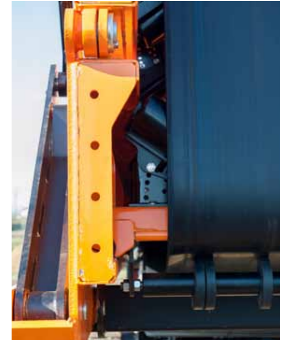
The ability to change the angle of rollers supporting the belt to form stream of transferred material (change of the belt's profile)
