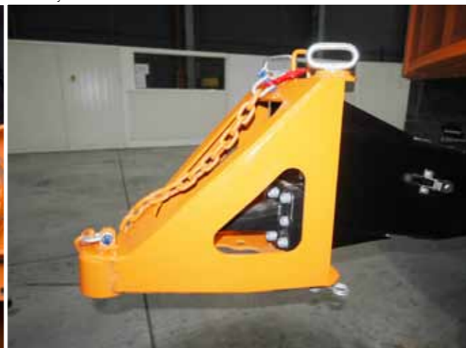
Ball coupling enables repositioning of the shredder using construction machinery.
