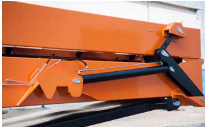
Stockpiler opening mechanism
