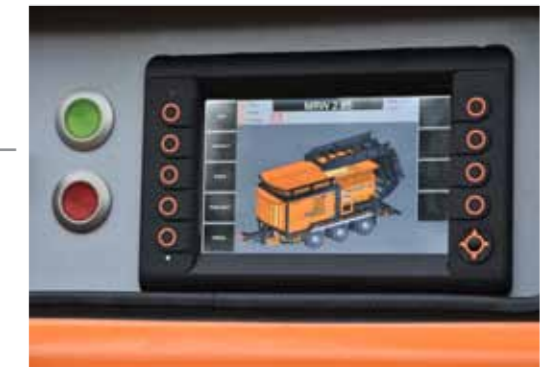
Central control panel with touchscreen
