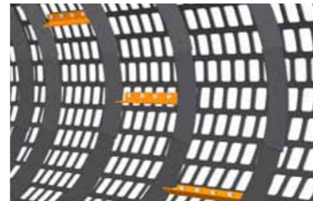
Steel lifters in the drum help more efficient separation and screening
