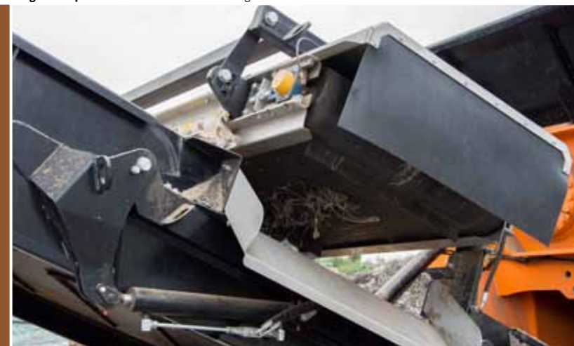
Magnetic separator for extraction of ferromagnetic materials.
