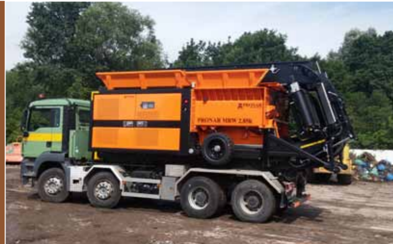
MRW 2.85h - carrying by hooklift frame carriers
