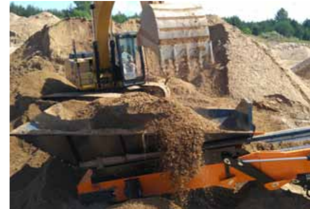
High durability of the stockpiler enables the use of a direct charge hopper with a capacity of 8 m 3 without any additional modifications to the stockpiler
