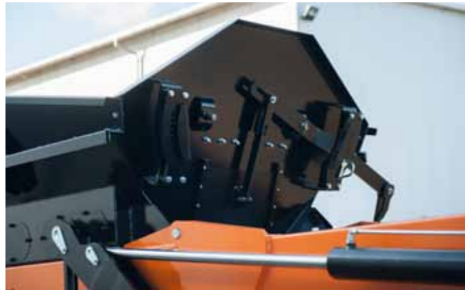
The hopper chute allows to adjust the release speed of the material from the hopper
