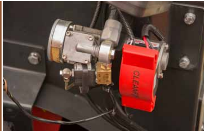
When working in difficult conditions and high dust content, in order to ensure the reliability of the engine and hydraulic oil cooling system, the radiators have been equipped with an automatic cleaning system (Cleanfix)
