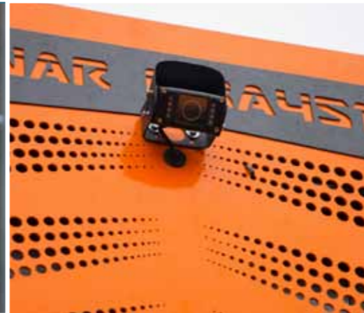
The camera ensures visibility on the back of the Windrow Turner, making it easier to work and raises the level of security
