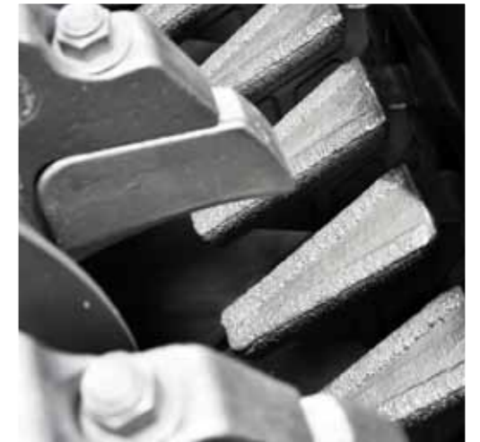
Counter knives. The grinding system tilting beam system with counterknives ensures long operations of the shredder allows removal of large, unbreakable materials - longer and troublefree operations of the machine. The standard electric reverse allows you to rotate the shaft in any direction without starting the combustion engine to remove blockages
