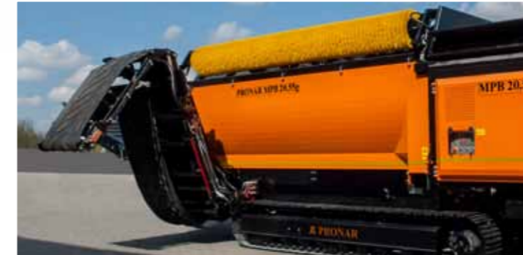
Conveyors retract to the outside of the machine - this allowed for lesser height
