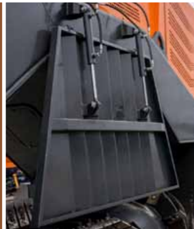
Adjustable tailgate limits the ejection of compost
