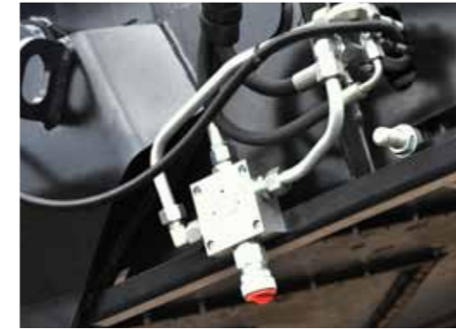
Conveyor belt speed rate adjustment
