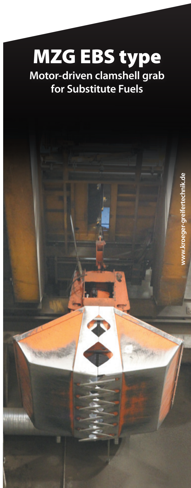
◀ Typ MZG EBS Motor-driven clamshell grab.
