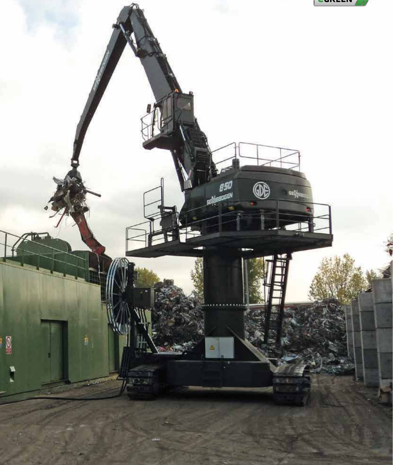
850 R special electro - with orange peel grab - loading of a scrap shear; France
