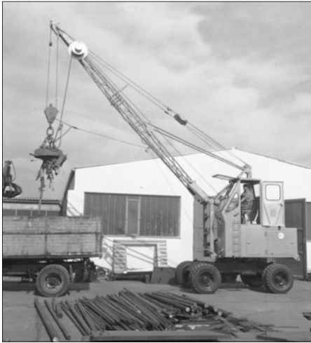
1962: rope-driven S833 with elevated operator cab
