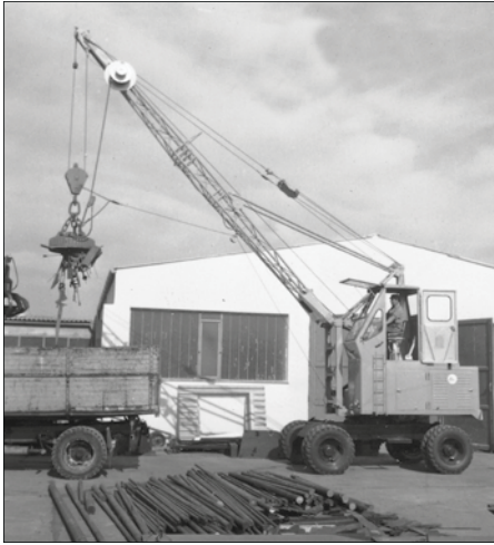
1962: Rope-driven S833 with elevated operator cab
