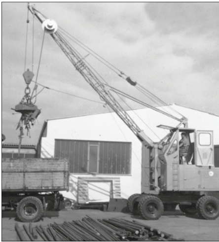
1962: Rope-driven S833 with elevated operator cab
