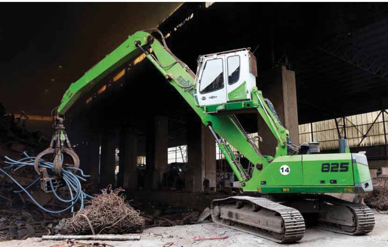
825 R - sorting copper scrap with original SENNEBOGEN orange peel grab; Turkey
