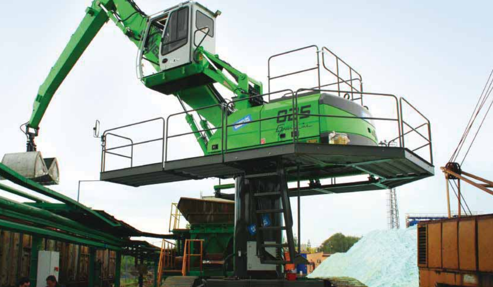
825 R - safe working in heights thanks to railings at upper carriage
