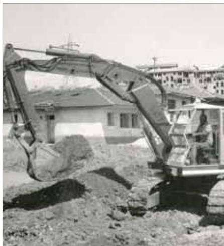
1976: S 517 with crawler chassis and plastic cab in earth moving
