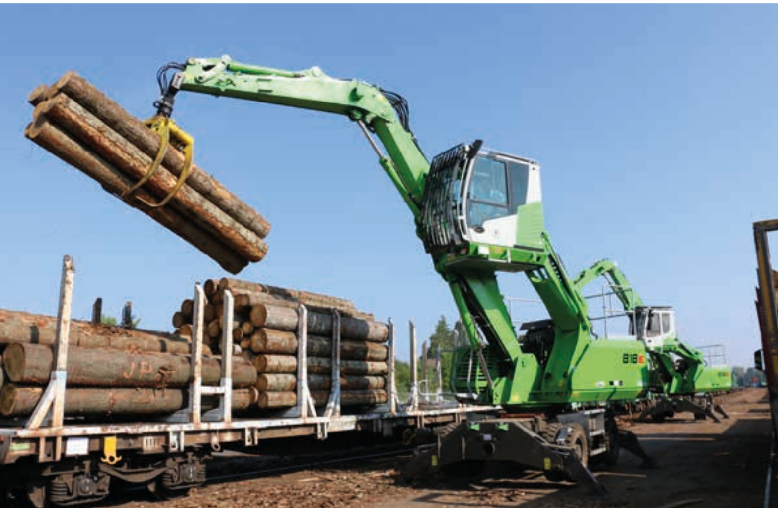
818 M - best overview when loading and unloading trains due to stepless cab elevation
